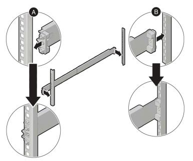
**a.** Snap the front slide-rails into the front rack posts.
