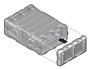
3. Secure the end-cap by latching eight wing-turn latches (turn clockwise, then close).
