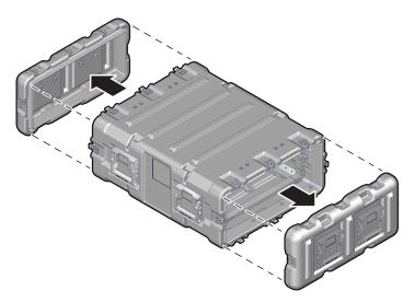
**4.** Remove the cable pouch, and extend the end-cap hooks.
